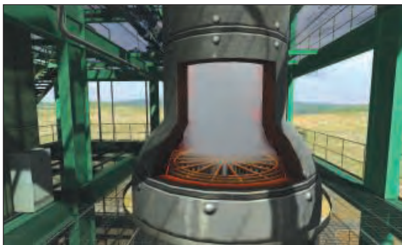
FIGURE 2. This image shows the transparent view of a gasifier operation from IGCC 3D, virtual immersive-training system
