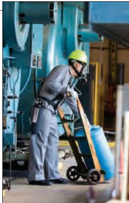
FIGURES 4a and 4b. Supplied-air respirators are designed to provide breathable air from a clean air source other than the surrounding work atmosphere. They include self-contained breathing apparatus units (left) and air-line respirators (right)
